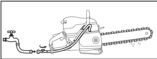
Attach to water supply capable of delivering 1.5 bar (20 psi) pressure to the saw at a minimum flow rate of 4 lpm (1 gpm). The single most important factor an operator can control to increase chain life is to use adequate water pressure.
