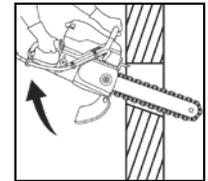
4. Pull saw out, rotate rear handle down, press bottom of saw to leading edge of cut and rotate rear handle up
