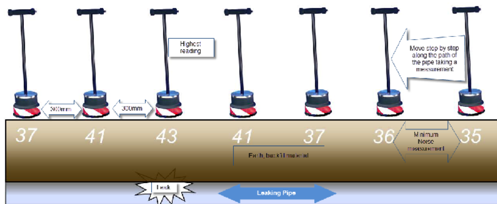
Fig.23 Method of Pin Pointing with a Geophone
