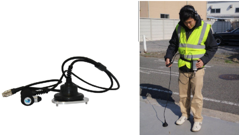
Fig.28 Pocket Mic as a Ground Microphone
