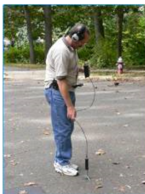
Fig.14 using the tripod attached to the hand probe microphone
