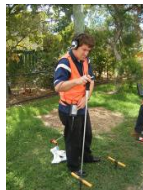
Fig.11 listening to the pipe via an insulated toughened probe
