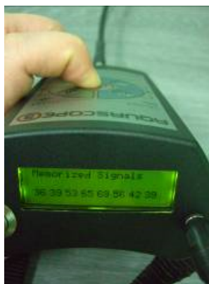
Fig.32 M button pressed and the last 8 readings displayed
