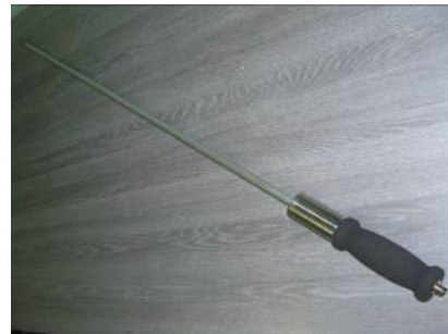
Fig.6 Hand probe Assembly using 2 x rod sections
