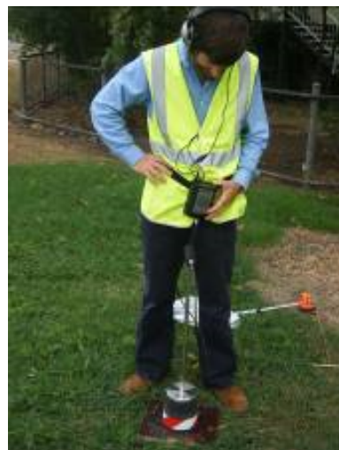
Fig.20 sounding using the Geophone on grass with a wooden board
