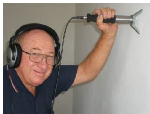
Fig.15 listening to a leaking pipe through the wall
