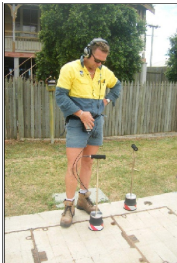
Fig.19 sounding using the Geophone concrete
