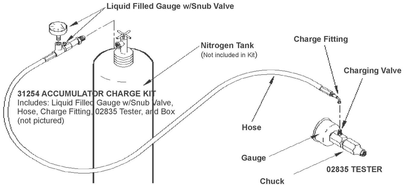
Charging the Accumulator Anti-Vibration Handles
