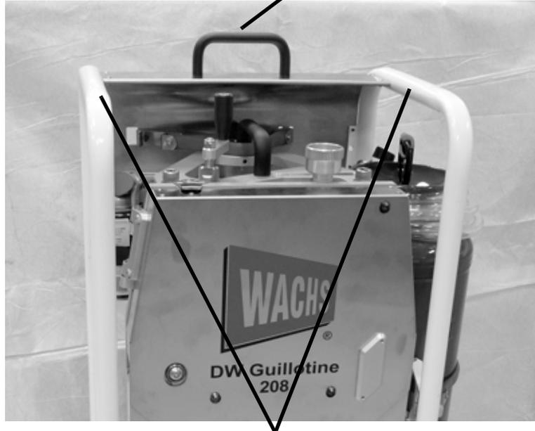
*Lift the cart by the frame tubes—one
