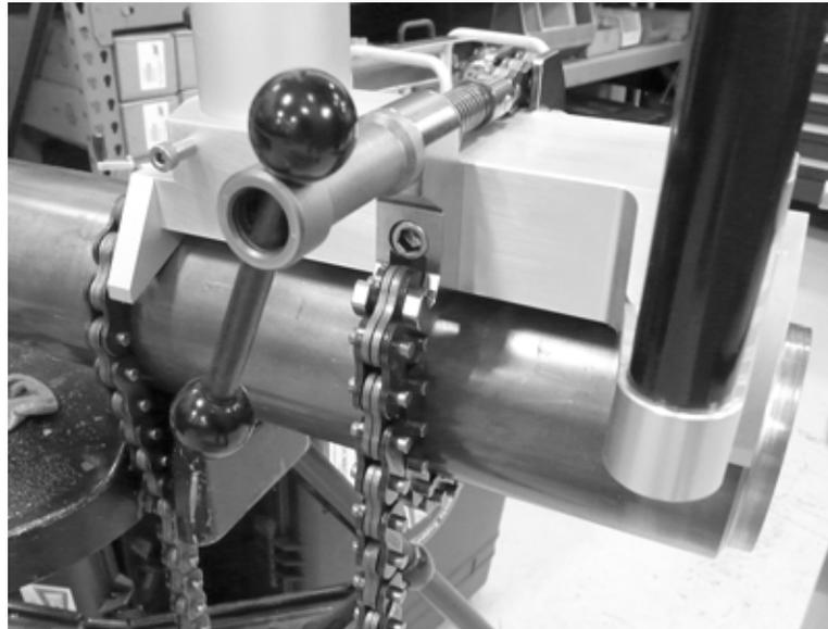
*Figure 3-25. Set the machine on the pipe, with the wire on the fall-off side of the cut.*
