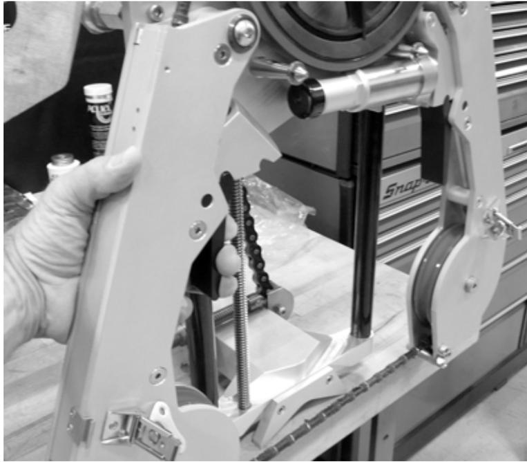
*Figure 3-22. Pull the left arm assembly to the open (operating) position.*
