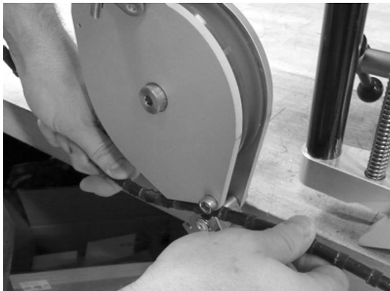
*Figure 3-19. Insert the cutting wire between the covers and the idler wheels.*
