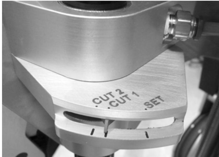
*Figure 3-32. Turn the feed handle to keep the tension gauge at the CUT 1 position for normal pipe, or CUT 2 for heavy-wall pipe.*
