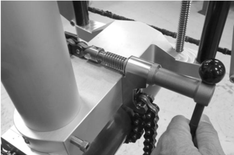
*Figure 3-26. Wrap the chain around the pipe and insert the link pins into the yoke as shown. Turn the handle to tighten the chain.*
