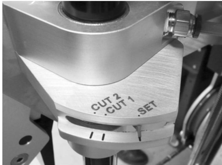
*Figure 1-6. Refer to the wire tension gauge to set the tension and operate the saw.*
