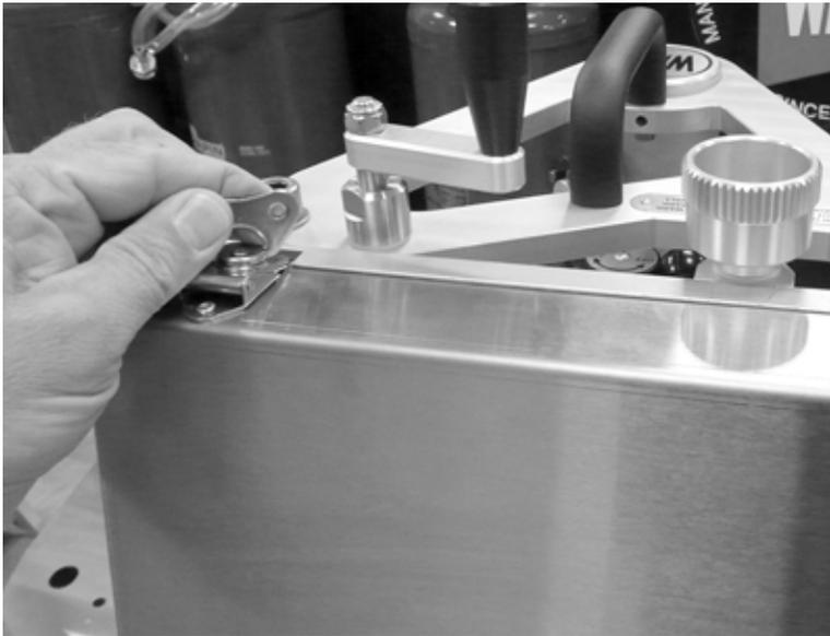
*Figure 3-24. Close the front cover and secure it with the latch.*
