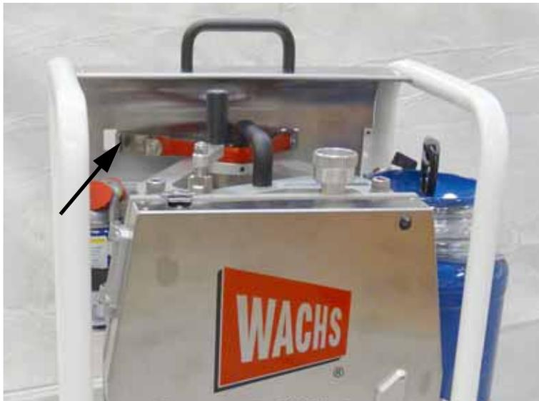
*Figure 3-1. Disconnect the storage strap to remove the saw from the cart.*
