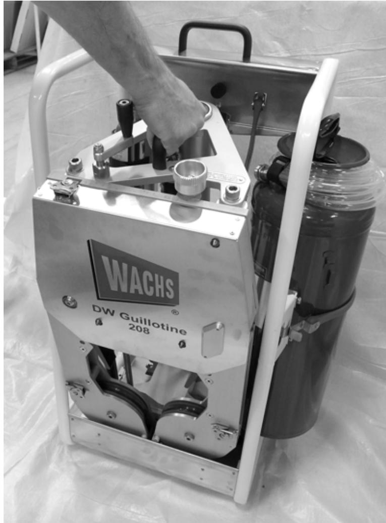
*Figure 3-2. Lift the saw out of the cart by its handle.*
