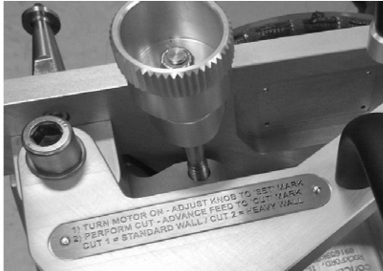
*Figure 3-13. A cutting instruction label is attached to the top of the saw frame.*
