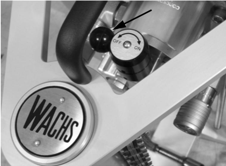
Figure 3-30. Make sure the ON/OFF knob is in the OFF position, as shown, before connecting power.
