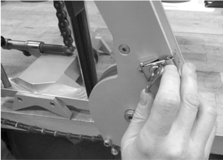
*Figure 3-8. The wire channel covers on the arm assemblies are secured by locking latches. Release the latch and swing the cover open to remove or install the cutting wire.*
