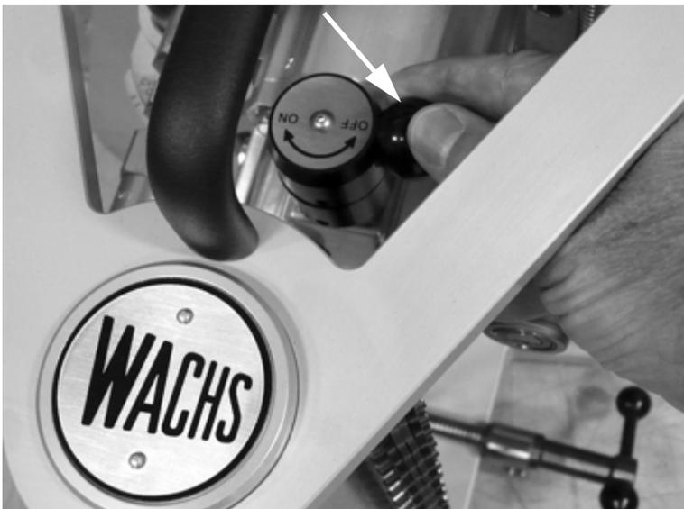
Figure 3-31. Turn the ON/OFF knob to the ON position to start the saw.
