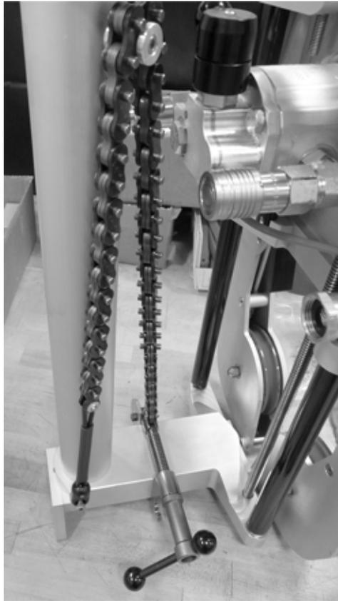
*Figure 3-33. Secure the clamping chain in its storage position, as shown.*
