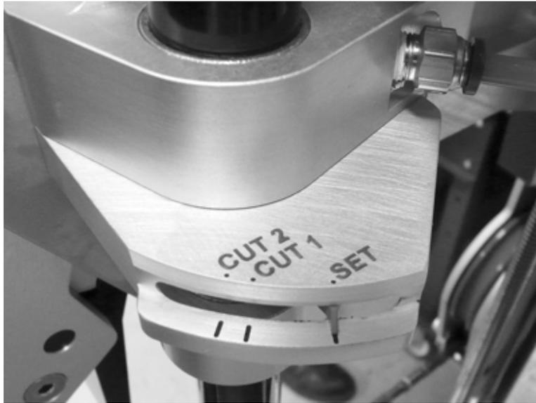
*Figure 3-28. Adjust the wire tension knob to set the tension gauge to the SET position.*
