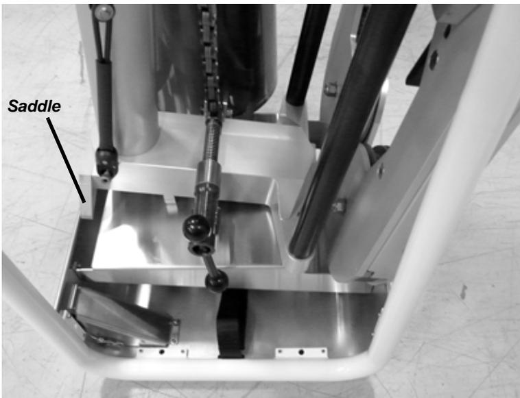
Figure 3-4. (Side view) Set the saw onto the brackets, with the saw saddle behind the cart base, as shown.
