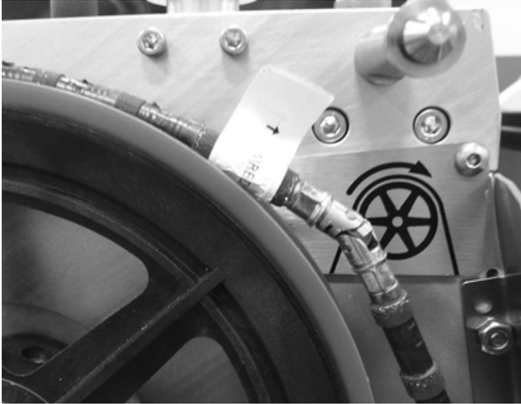
*Figure 3-17. New cutting wires have a label indicating the cutting direction.*
