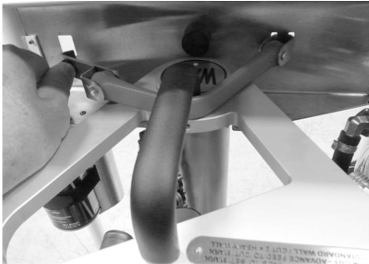
*Figure 3-5. Secure the saw to the cart with the storage strap.*
