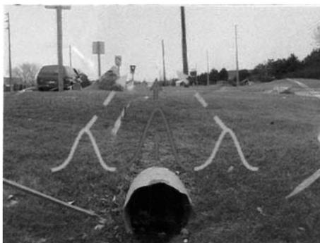
Culverts like other large metal objects send out interfering ferrous signals which could be interpreted as the Culvert. The (TID) function will identify these false signals with a the **Mode Tone & Green LED**.
