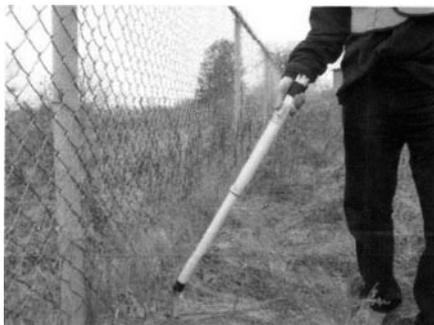
Hold locator at a slight angle to fence. A **Mode Tone & Green LED** will appear. Next move Locator along the fence line. When a strong **Audio Tone & Red LED** appears this will indicate a possible Vertical Target Object.
