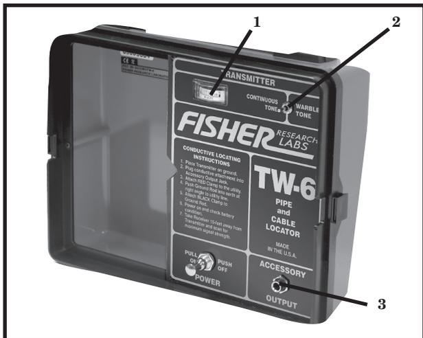
**3. Accessory Output:** The Ground Plate Assemblies Coupling Clamp or Ground Rod Assembly connects into this jack for a Conductive Trace or Direct Induced Trace.
