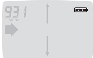
3. **Left/Right & Over-Target:** These indicators show your position relative to the center of the electromagnetic field.
