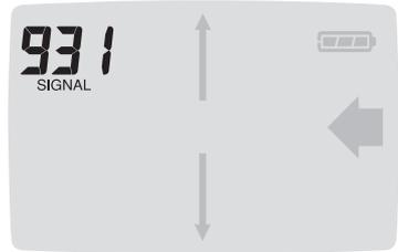
2. **Battery Strength:** When battery life declines to less than 1 hour (estimated) of operation the battery indicator outline will be illuminated with no segments. When the batteries reach the end of their useful life, the screen will go blank and the battery icon will flash before the Receiver shuts off. Expect about 60 hours of battery life from a set of two D-cell alkaline batteries.
