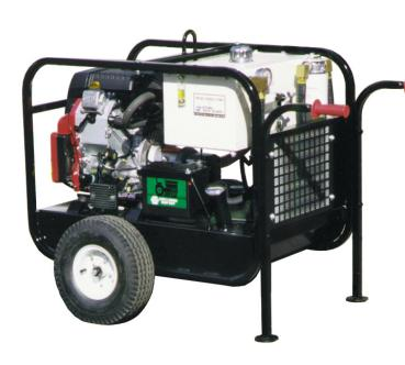
This power unit features a 22 HP Honda OHV gas engine, extended run fuel tank, extra oil cooling and easy handling. It is available with a fixed displacement gear pump or pressure compensated piston pump. Great for continuous duty applications powering our pumps or other hydraulic tools and equipment. Variable speed throttle controls hydraulic output.
