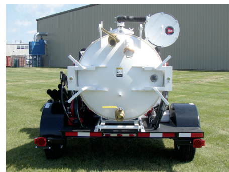
The heavy-duty spoils tank features a two-cylinder electric over hydraulic slide, tilt and dump functionality for easy emptying
