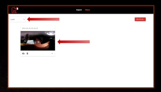
Use the dual-ended USB that was provided with your RV-MAX 360 to transfer the videos from the tablet to your work computer. Note also that RinnoView can be installed to any other computer if you'd like to improve the workflow by avoiding this step. Contact RinnoVision or your local distributor's technical support if you're interested and we'll gladly help you set this up.
