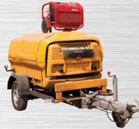
A hydraulic Power pack on top of an Air Compressor, both sized to operate the same rated Breaker.
