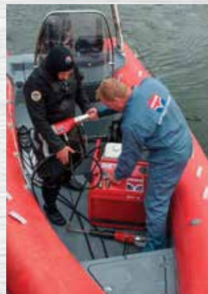
A hydraulic Power pack on top of an Air Compressor, both sized to operate the same rated Breaker.
