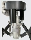
4. Hand tighten the light kit mounting nut.
