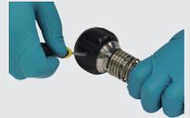
2. Slide the camera head into the skid barrel until the head is flush with the front of the skid.
