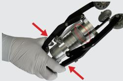
2. Turn the diameter adjustment nut counter-clockwise to increase the diameter of the skid or clockwise to decrease the skid diameter.
