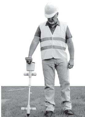
**Position of Receiver for Tracing**
