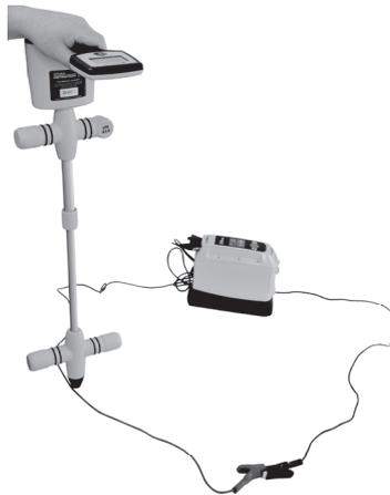
Configuration for Testing the Conductive Attachment
