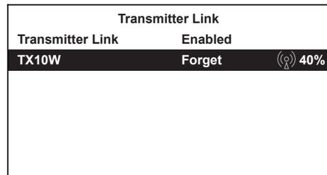
7. The "Beacon" icon on the transmitter should not be flashing anymore at this point. A solid icon indicates that the link has been established.
