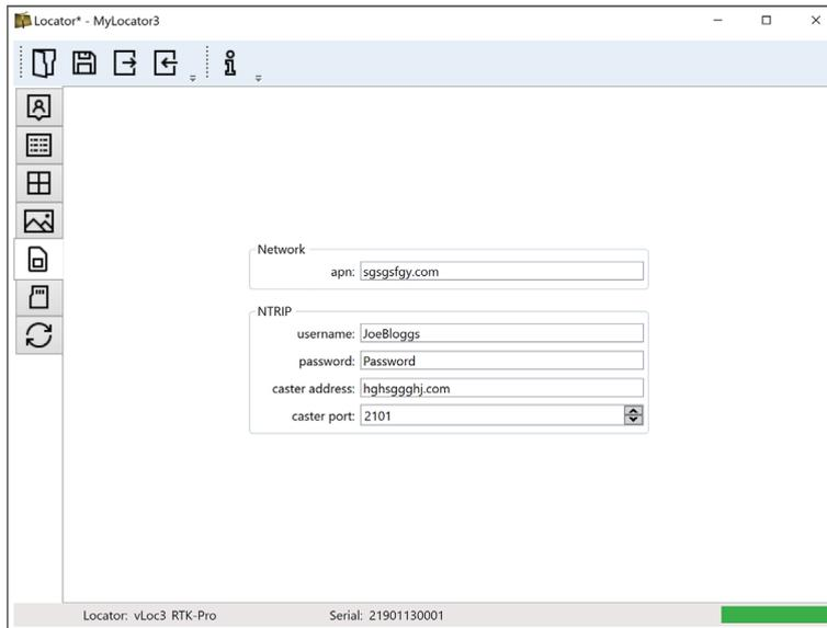
4. **Network "apn:"** should be adjusted to the Access Point Name for your chosen Mobile network – be sure not to add any spaces before or after the APN. If you do not have the APN, it should be possible to do a quick web search on "APN settings for a mobile network."
