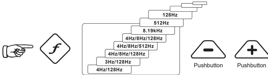
As with most manufacturers, signal clamps are tuned to specific frequencies and **will not** work over the complete range of frequencies
