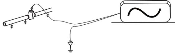
Unlike passive detecting, active locating has the benefit of the operator controlling the signals and can be more specific about what line is detected. Passive signals are also not always present on a line, so using active signals ensures more lines are detected.
