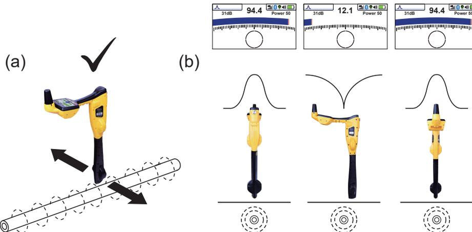
7. Rotate the vLoc3 RTK-Pro on its axis to obtain the maximum signal. The vLoc3 RTK-Pro is now directly over the line and with the blade across the line. (If using the Omni-Peak mode, there will be no change so switch to Peak mode if the direction is required).
