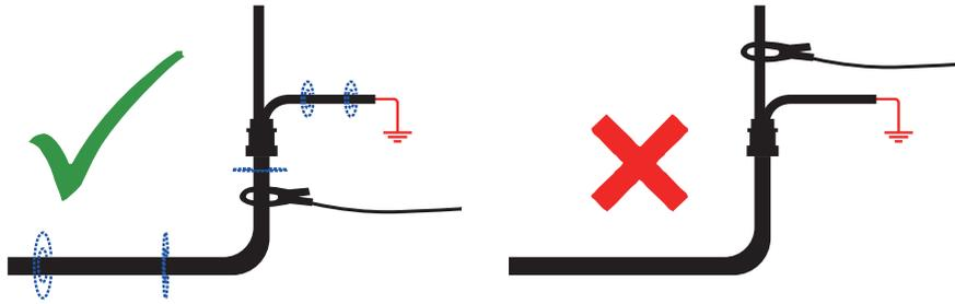
When applying a clamp close to a grounding point where multiple grounds or a grounding bus exists, ensure that you place the clamp around the target line and not to the ground bus/other grounds. This will help focus the applied signal on the target line.
