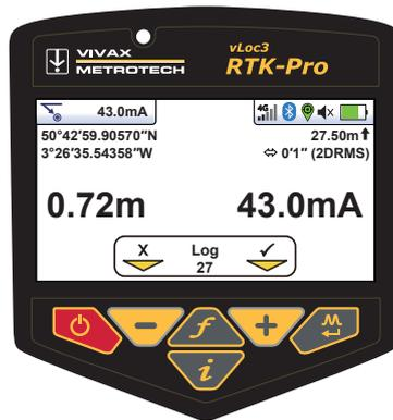
When in a Locate screen, a quick press of the “i” (information) pushbutton will display the depth and signal current.
