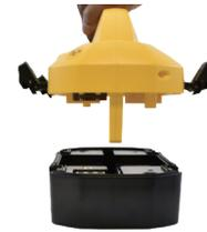
3. Lift the transmitter base from the battery tray.
