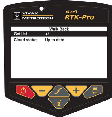
2. At the **Get list** option and press the enter pushbutton to bring up the list of Walk Back points allocated to this receiver's serial number from the VMMMap Cloud.
