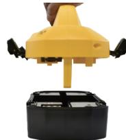
1. Align the aligning post and lower the transmitter base into the battery tray.
