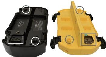
The battery tray and transmitter base have a matching aligning post, contact pins and socket.
