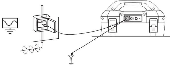
Wherever a direct connection can be safely made without the risk of injury, damage to the customer's plant, or the transmitter, it is the best way of applying the transmitter's signal.
