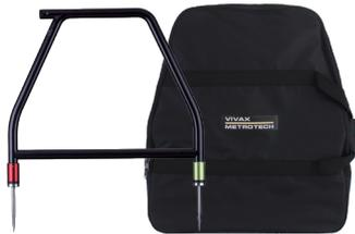
The A-frame accessory is used to detect ground faults on pipes and cables. In the case of pipes, the faults consist of coating defects. In cables, faults are usually caused by insulation damage allowing the metallic sheath (or internal conductor) to contact the earth.
