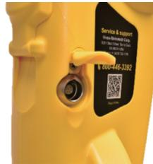
Connect the charger to the charging/accessory socket of the receiver. Connect the charger to the mains and switch it on. The LED indicator on the charger will illuminate red until the batteries are fully charged, at which time the LED will change to green.
