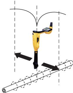
The Delta Null has the advantage that it provides a sharper response than the "null" mode and is less affected by distorted fields. All other functions are the same as the "Null" mode.
