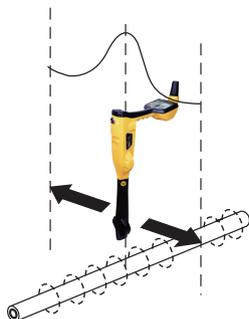
The Peak with Arrows mode operates in the same way as the peak mode. It gives the largest meter deflection when directly over the line. However, the left/right indication arrows are also displayed. The arrows indicate the direction to move the receiver to locate the position of the buried line.
