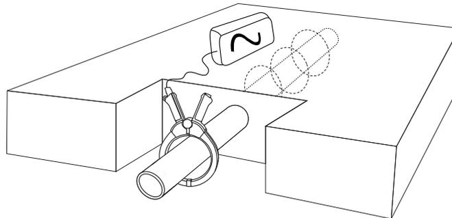
In many situations when it is not possible to make a direct connection to a cable, a signal clamp will provide an efficient and safe method to apply a locate signal.
