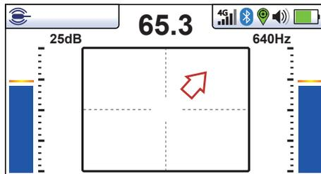
6. If the bar graph is not steady, it will most likely be because the sonde is not within range. In this case, hold the locator at approximately 45 degrees to the ground and rotate the locator around a full 360 degrees around you. Note the strongest signal's direction and walk towards it until the bar graph shows a steady signal. Now revert to step five above.
