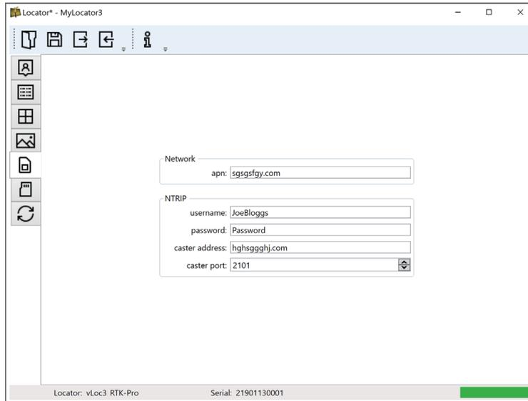
“Network” “apn:” should be adjusted to the Access Point Name for your chosen Mobile network – be sure not to add any spaces before or after the APN. If you do not have the APN, it should be possible to do a quick web search “APN settings for a mobile network.”
