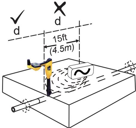
Also, note that the signal will radiate out to the sides and below the transmitter. For this reason, it is recommended that when applying a signal using the induction method, a distance of at least 4.5m (15-feet) is kept from the transmitter when pinpointing or taking depth readings.
