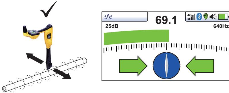
Hold the locator vertically and rotate it on its axis until the compass indicates Forward/Back, as shown above.
