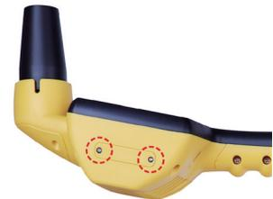
The SIM card slot is positioned between two micro USB sockets. The USB sockets are used in manufacturing only so they should be ignored.
