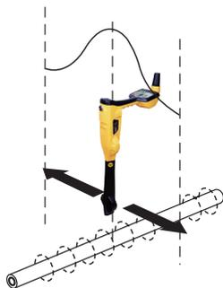
Two horizontal antennas provide a “Peak” or maximum signal response over the buried line.
