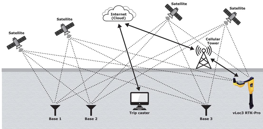
This set-up procedure assumes the operator has a suitable data-enabled SIM card registered with a cellular network provider and that the operator has registered with an RTK provider. It is also assumed that the operator has the latest version of MyLocator3 installed on a computer. (see the section on MyLocator3).
