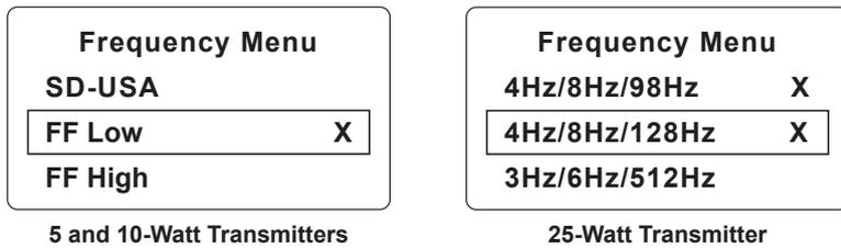
5. After selecting the frequencies press the “i” pushbutton again to exit the “Frequency Menu” and return to the main display.
