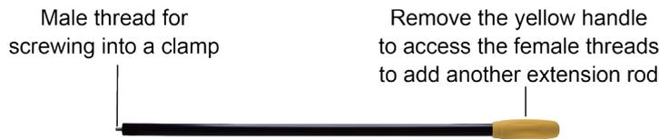
The extension rod is fitted with a 10mm threaded male stud. This male thread screws into the handle of the signal clamp to extend the distance of the clamp. This helps areas with difficult access, such as in manholes or trenches. (not to be used on uninsulated overhead power cables).
