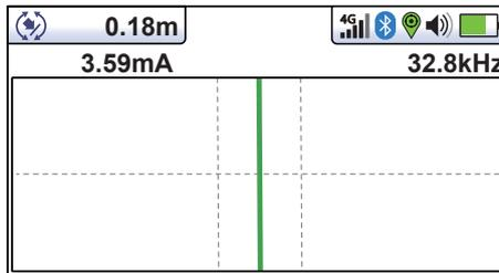
"Tram" lines on either side of the line indicate an area of confidence. The closer the tram lines are together, the greater the confidence.
