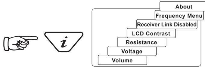
When the “i” (information) pushbutton is pressed, the display will show the volume level. Use the + and - pushbuttons to increase, reduce or turn the speaker off. (off-low-medium-high).
