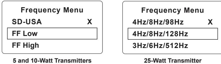
3. Pressing the “+” or “-” pushbuttons, you can scroll up or down through the available frequencies.
