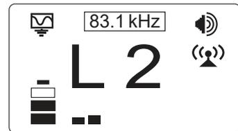
5. While the icon on the transmitter is flashing (indicating that it is waiting to connect to a receiver), switch on the vLoc3 series receiver and enter the user menu by pressing and holding the information button. Scroll down the menu options until Transmitter Link is highlighted.
