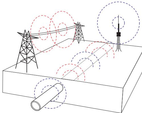
**Radio signals** - Low-frequency radio transmitters create radio signals. These are used for broadcasting and communications and are positioned throughout the world. As the frequencies are very low, the signals tend to penetrate and hug the earth's curvature. When the signals cross a long conductor such as a pipe or cable, the signals are re-radiated. It is these re-radiated signals that the Radio mode can detect.
