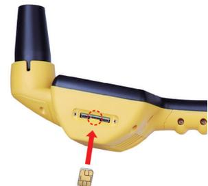
To remove the nano-SIM card, push the SIM in to unlatch it before it is released.
