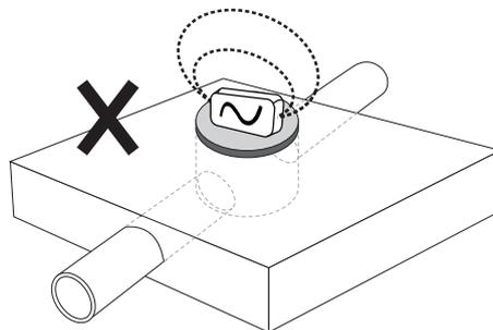
When using the induction mode, avoid placing the transmitter over metallic manhole covers. Doing so will severely reduce the transmitter's effectiveness and, in extreme cases, cause damage to the transmitter's circuitry.
