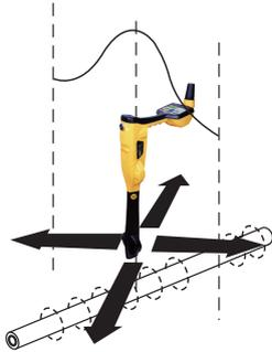
The two double-ended arrows around an icon mean that the line is detectable regardless of locator blade orientation.
