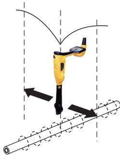
The vertical Null antennas receive a minimum or "Null" response over the buried line.
