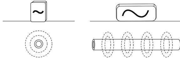
Remove all connections from the output connector. Switch on the transmitter and place it over the suspected position of the line and position it so that it is in line with the target. In the case of the Loc3 series transmitters, that is with the handle pointing along the line.
