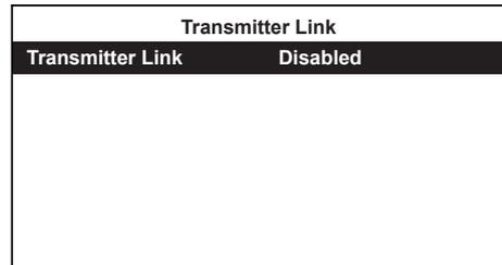
6. Select the "Transmitter Link." Check that the radio module is enabled. If not, press the return button to enable the Transmitter Link. After a short scan, the available devices will be displayed. Highlight the one to be selected and press the return button. Press the information button to return to the main menu.
