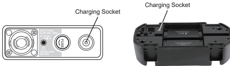
**Plug the charger into the charging socket on the side of the transmitter or directly into the battery tray**
