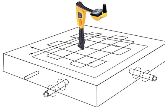
4. Keeping the vLoc3 RTK-Pro vertical, walk across the area to be checked, keeping the orientation so that the blade is in line with the direction of walking (See diagram above). If using the Omni Peak mode, the orientation of the locator is not important.
