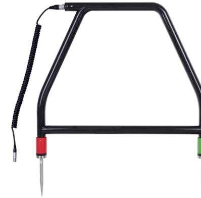
**Accessory A-frame – Plugs into the vLoc3 series receivers**
