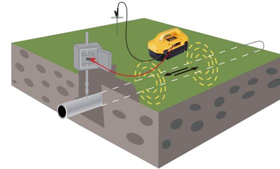
**Clamp** – induces a signal into a pipe or cable without making a direct connection
