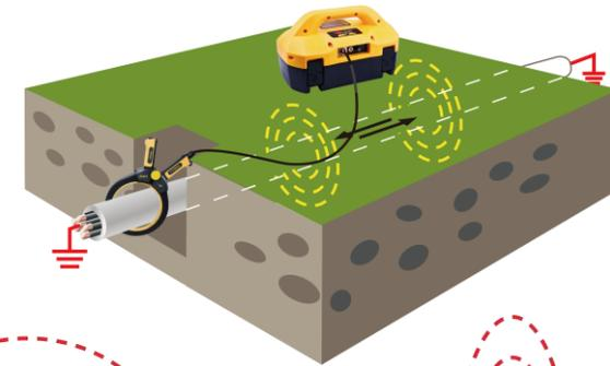
**Induction** – induces the signal onto a pipe or cable by placing the transmitter on the surface over the target line
