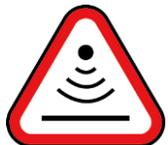
This indicates that the signal is mainly radiating from above. This is usually caused by the signal travelling along overhead cables.
