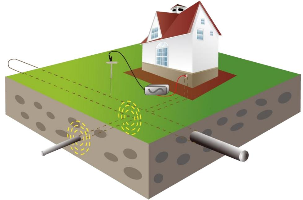
\* Tracing is following the path of the buried line from, or to the transmitter
