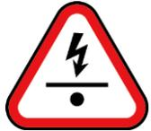
This indicates that the locator has detected a cable that is possibly less than 15cm deep. Proceed with caution.
