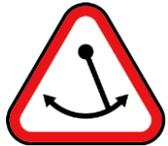
This indicates that the operator is swinging the locator excessively and could result in misleading information. When sweeping the locator across the direction of the line, try to keep it vertical. This will improve accuracy.
